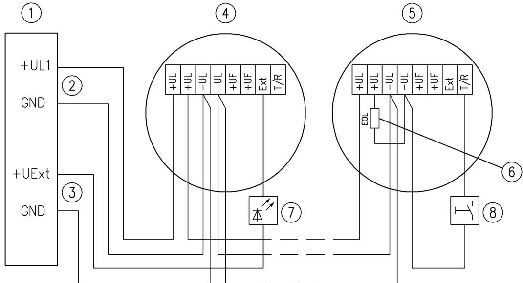
Fig. 36: Alarm line wiring diagram, external display and test/reset button
