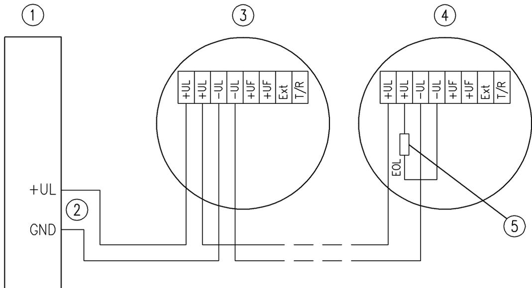
Fig. 34: Alarm line wiring diagram, without fault line
