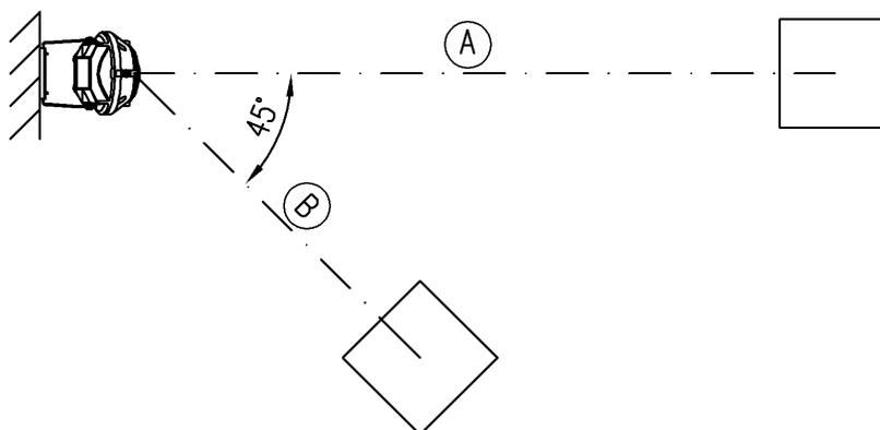
*Fig. 15: Sensitivity is reduced by half at an angle of 45°*
