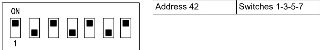
Fig. 43: DIP switches on KMX5000 AP
