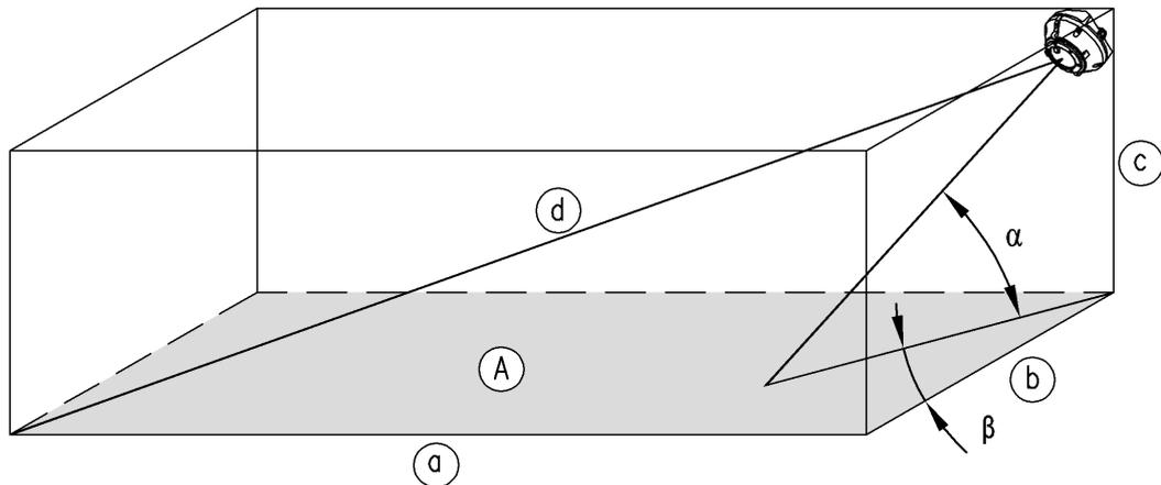
Fig. 14: Room monitoring as per VdS 2095: 2010-05 (07)
