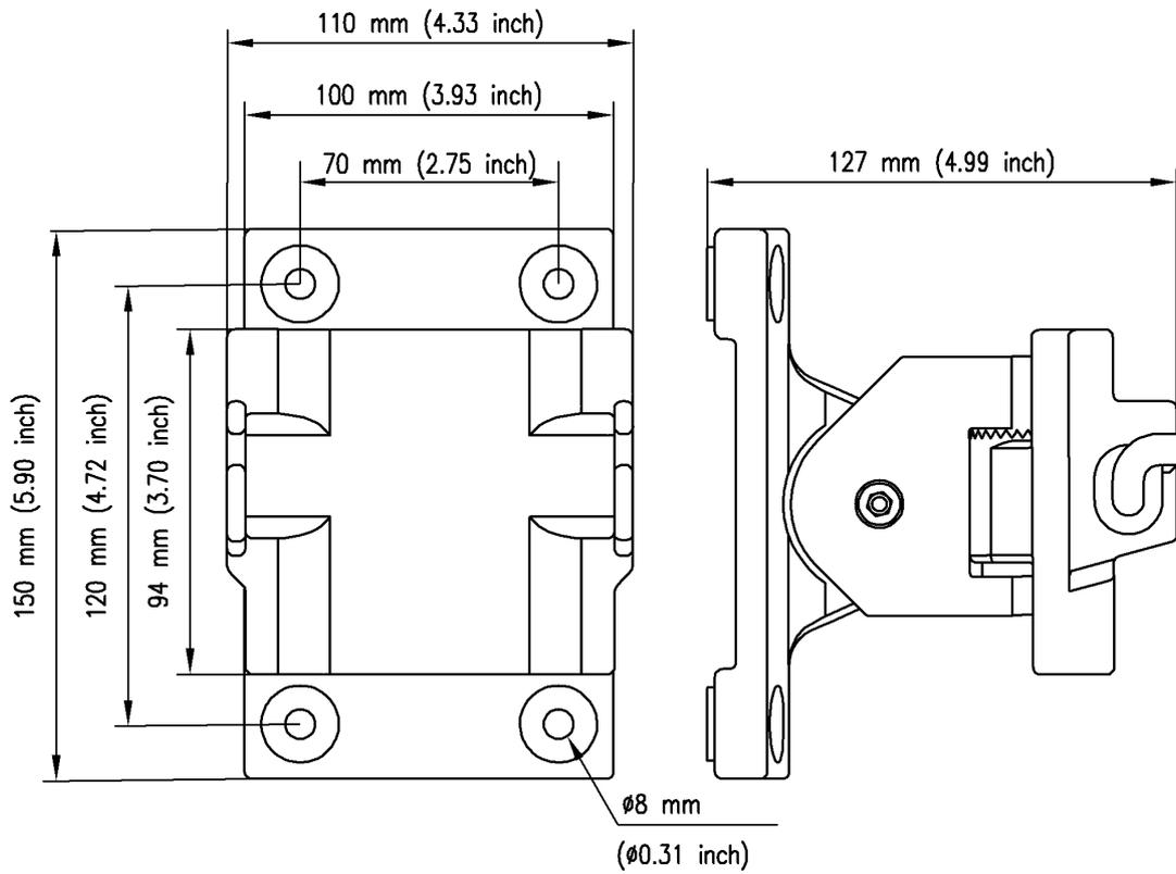
*Fig. 27: Assembly dimensions of MX5000 ST mounting bracket*
