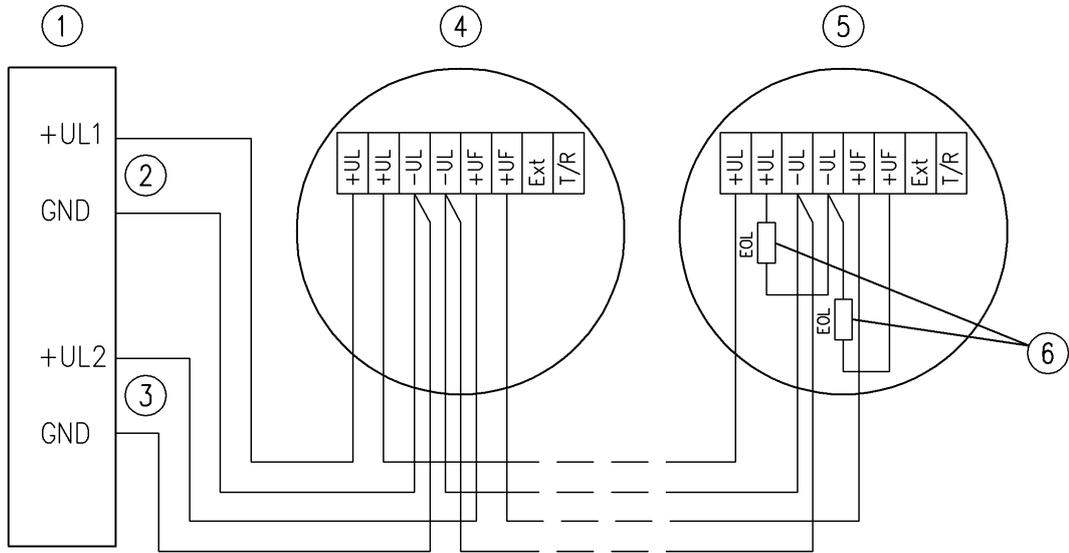
Fig. 35: Connection of alarm line to fault line
