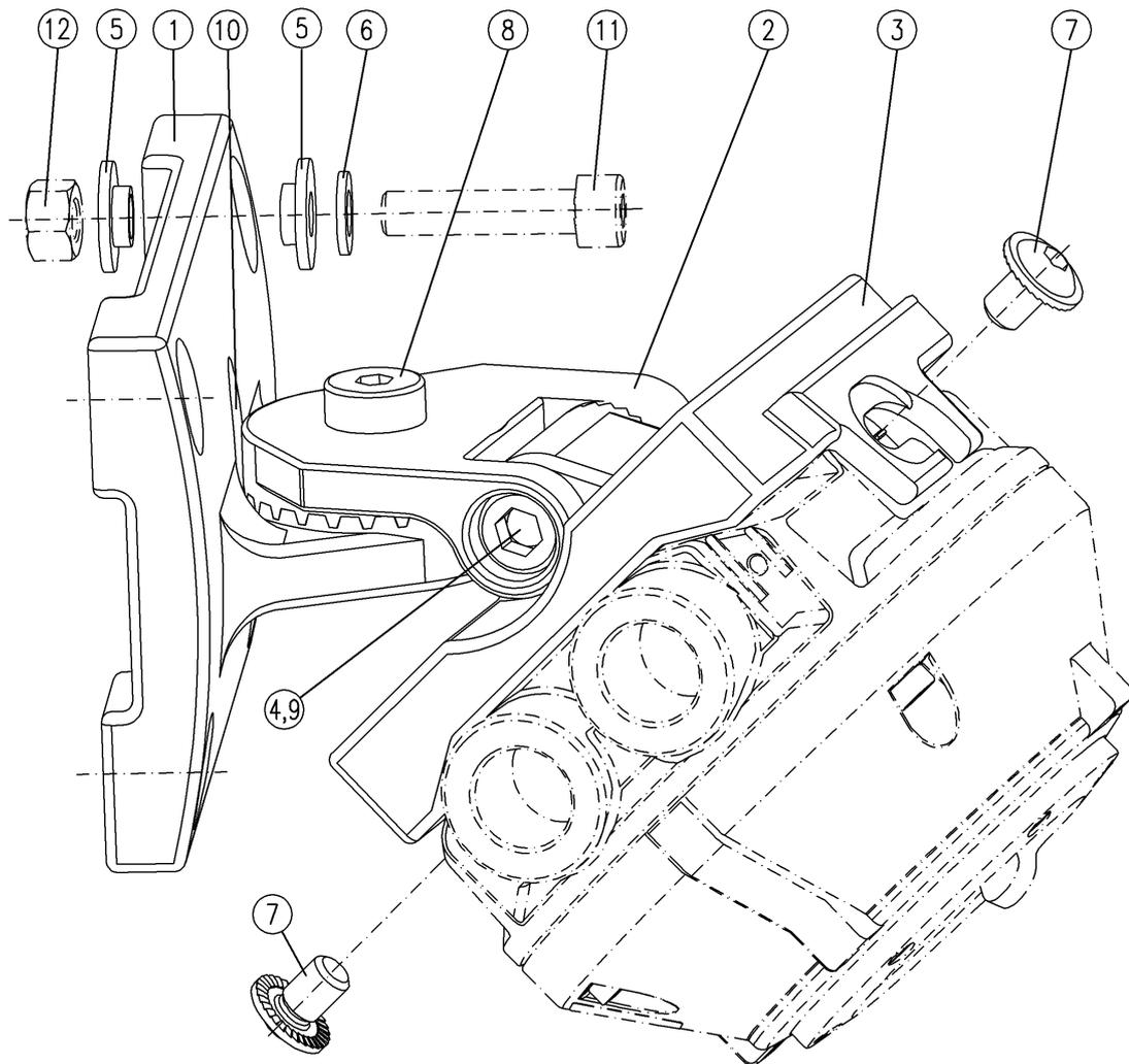
**Fig. 28: Assembly of MX5000 ST wall mounting bracket**
