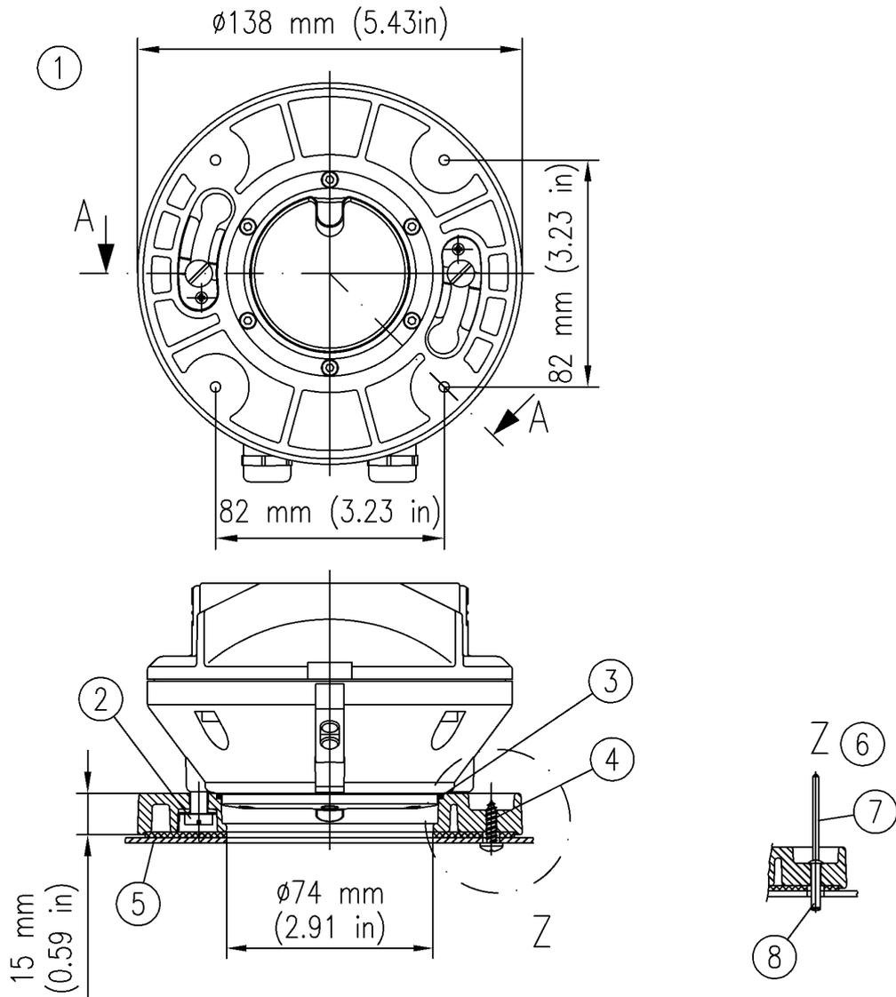
Fig. 29: Device and assembly dimensions for the bracket mount installation
