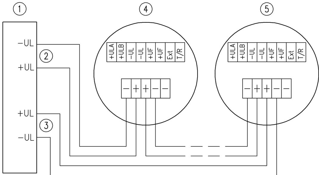
Fig. 42: Insulator base connection diagram
