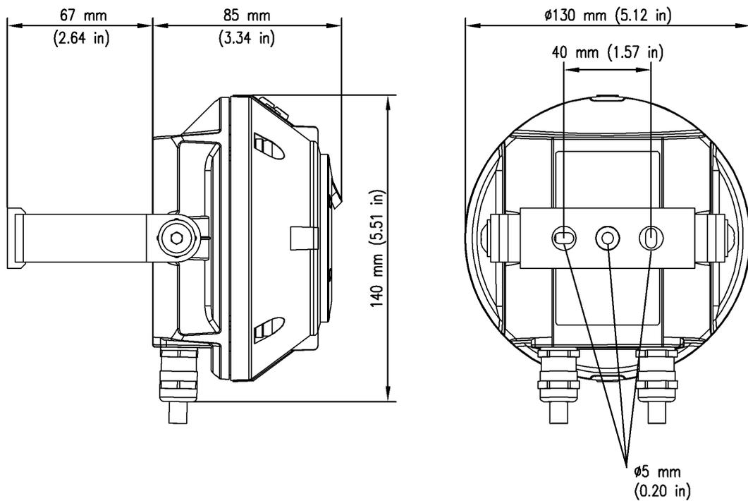
*Fig. 21: FMX5000 IR – Device dimensions and assembly dimensions for swivel mount installation*
