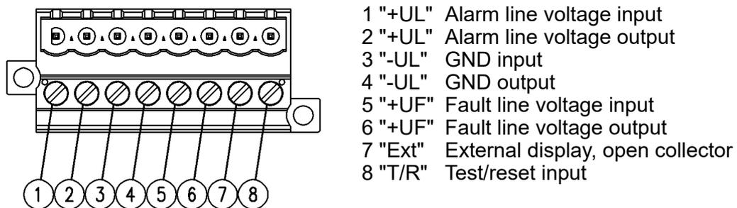
Fig. 33: Connecting terminal configuration
