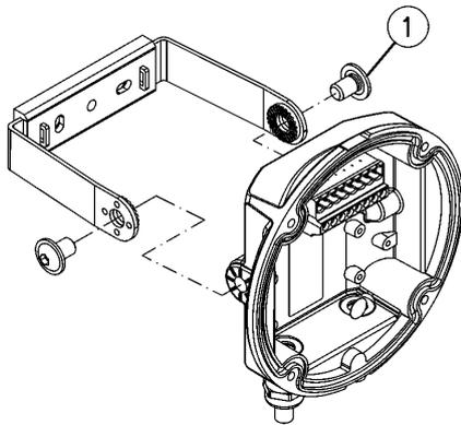
*Fig. 23: MX5000 detector base for swivel mount installation*
