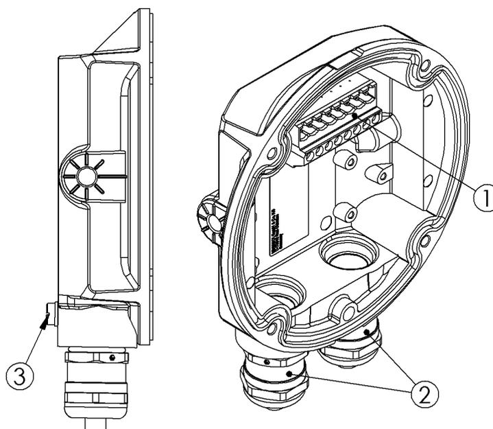
Fig. 9: Example, detector base MX5000 M20 Ex
