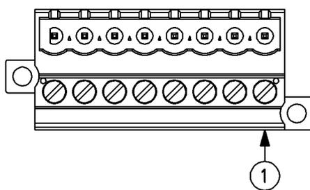
1 Test/reset input connecting terminal
