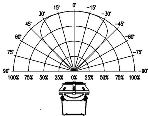
Fig. 4: FMX5000 IR and FMX5000 IR 3GD viewing range
