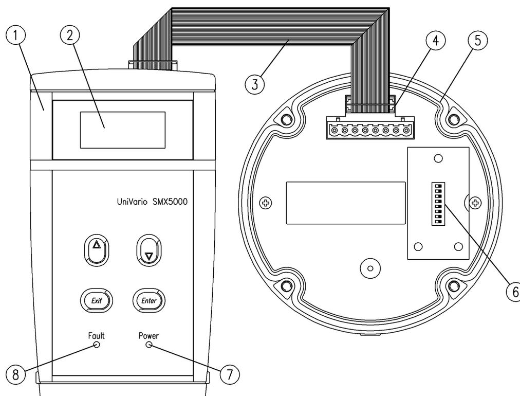
Fig. 17: SMX5000 connected to UniVario® detector
