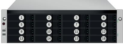
Figure 4.6: Drive slot numbering for 3U models
