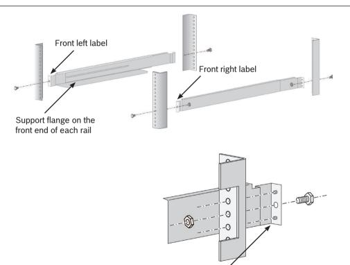
Guide pins on rails align with holes in the rack post
