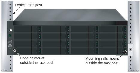
Figure 4.5: System installed in rack
