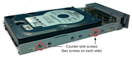
Figure 4.9: SATA disk drive mounted in a drive carrier
