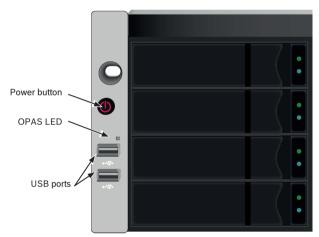
Figure 4.11: Front panel components on the left handle
