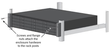
Figure 4.4: Secure to rack
