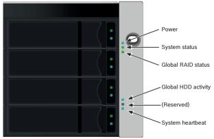
Figure 4.12: Front panel LEDs on the right handle
