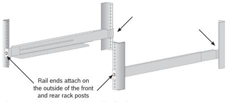
Figure 4.2: Rail ends attach to the outside of each post
