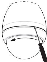
**Figure 14.44: Pendant Bubble Release Opening**
